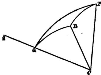
Let  $C$  denote the centre of the spheroid,  $CP$  the semi-axis of revolution,  $Q$  any point on the surface having for its polar co-ordinates  $s$  and  $\theta$ . Produce  $CQ$  to any point  $q$ . It is required to find the *horizontal* attraction on a particle at  $q$ . Let  $Cq = \delta$ .
